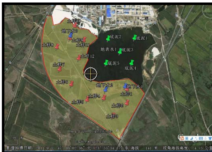
Locations of first sampling at the site; note that red stands for soil samples, blue for water samples and green for sediment samples; map capture by Mao Da
