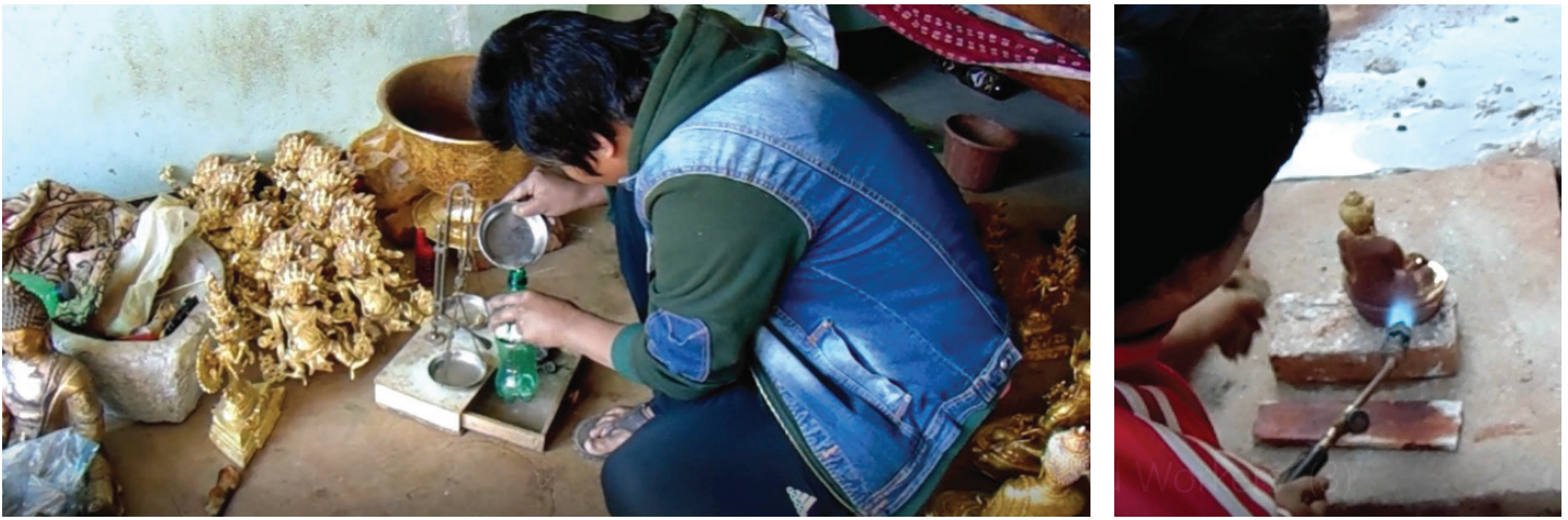
Figure 1. Nepalese plating workers applying mercury/gold paste to statues and burning it off with a blow torch. Source: CEPHEd
