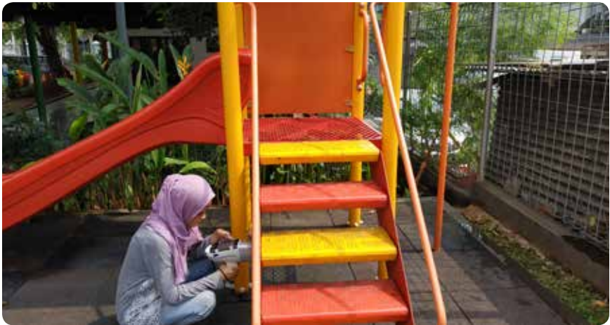
Figure 7. Staff of Nexus3 Foundation measuring lead content in playground facilities using portable XRF analyser. Photo: Nexus3 Foundation
