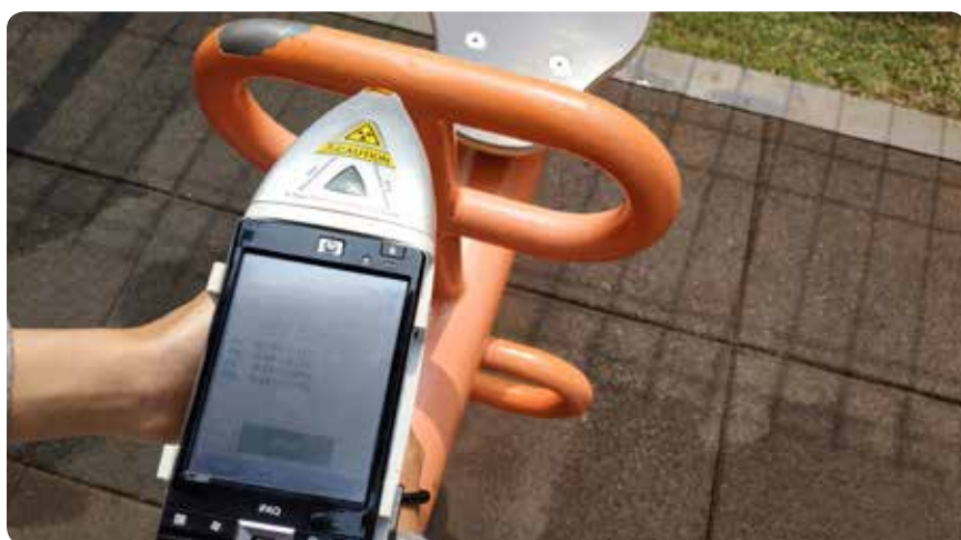
Fig. 3. (a) Yellow colour contained higher lead than other colour; (b) peeled off paint in accessible part of the play equipment is one of the source of lead exposures to children when they are playing. Photo: Nexus3 Foundation
