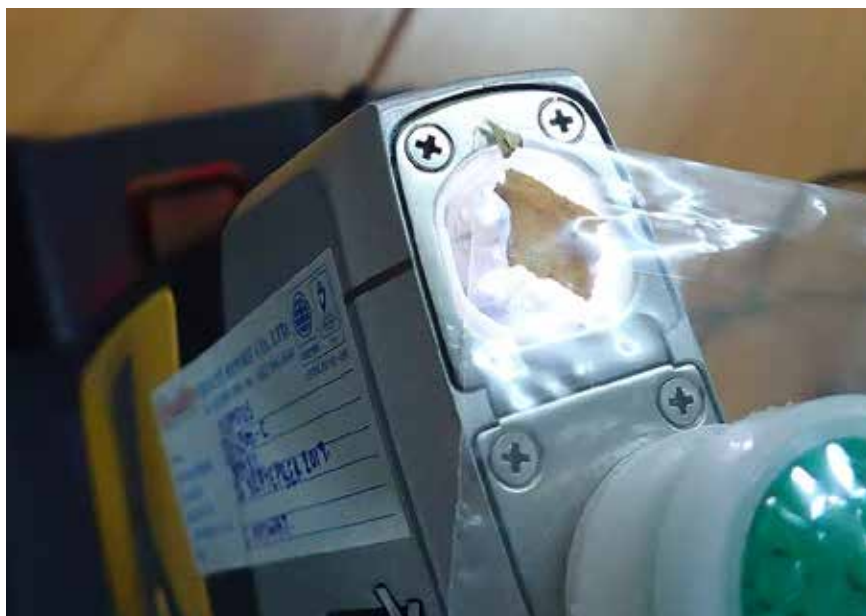
Figure 1. Photo of staff of CAP measuring lead content in paint chips obtained from playground facilities using portable XRF analyzer.
