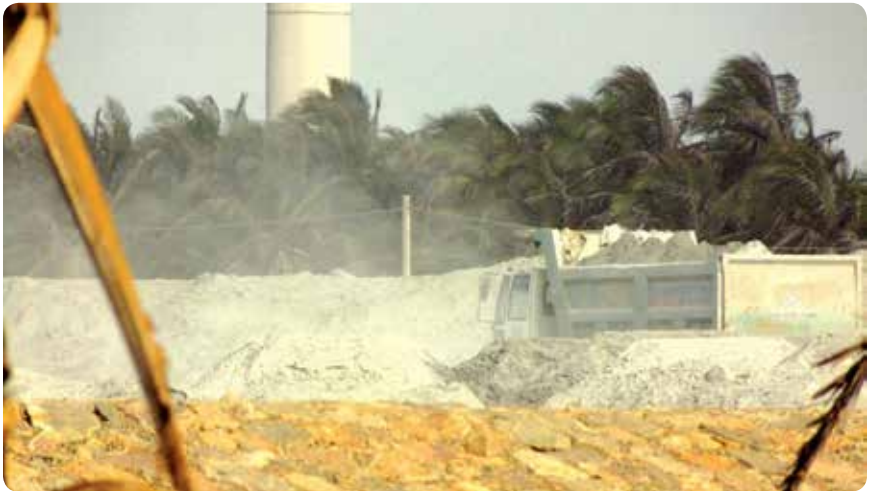
Figure 17. Poorly controlled ash from the coal-fired power plant is blown into the air during strong winds. Source: The Sunday Observer, Sri Lanka
