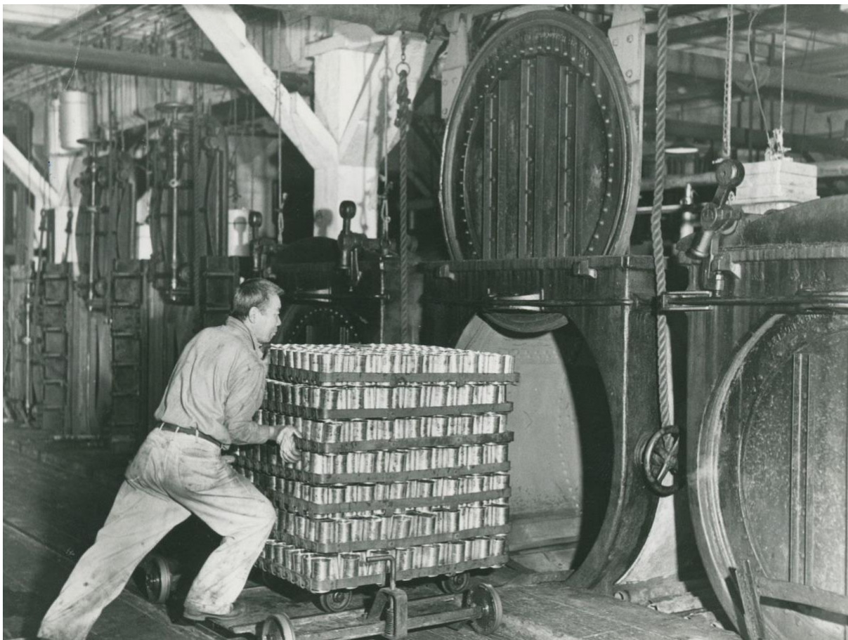
Figure 11: A worker slides trays loaded with one pound cans into a retort for cooking. Retorts improved the consistency of cooking, allowing for increased production. Gulf of Georgia Cannery Collection CFC 3-19-3
