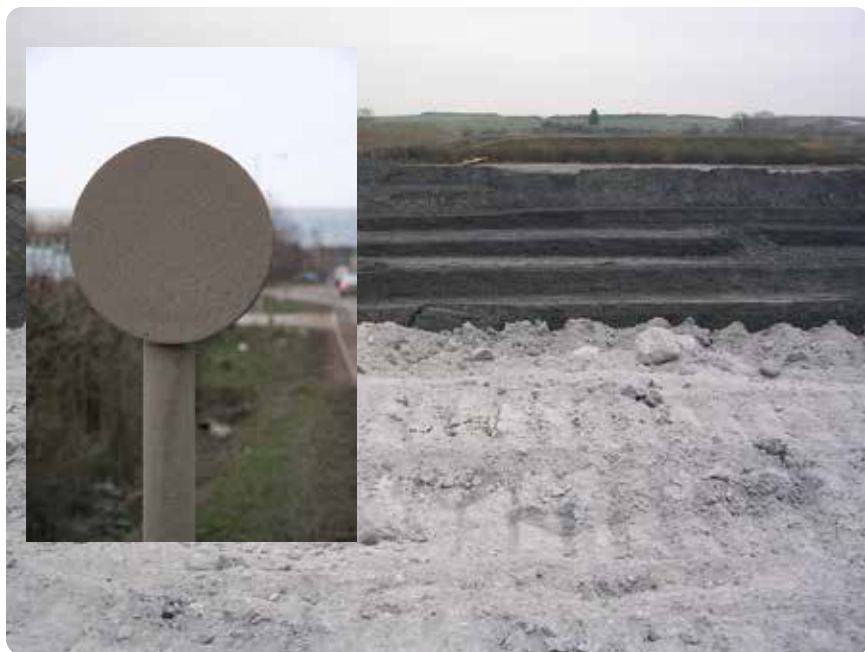
Figure 4: This picture shows the light grey surface of the APC residues in the Bishops Cleeve landfill, one of the fly ash disposal sites in UK. The inset picture shows a 40 mph speed limit sign at the side of the site access road. Source: Watson (2015).
