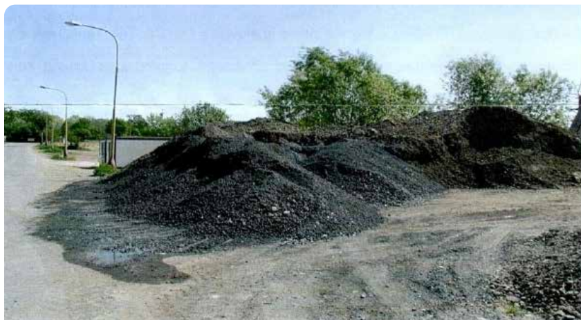
Figure 27: Interim storage of mixed fly ash and bottom ash from MWI Liberec, Czech Republic before its use as construction material in one of the municipalities. Levels of PCDD/Fs in this material are 0.05 - 0.1 ppb in WHO-TEQ. There used to be a prohibition not to dispose of fly ash any other way than at a hazardous waste landfill. It has changed since 2005.
